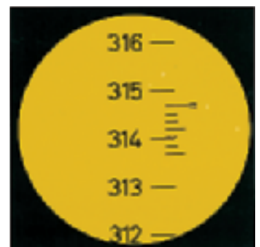
NAK2 circle reading (360°) 314°42'
